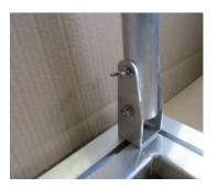
i) Stick ring nuts M 6 x 50 through boreholes of the net hoop (position see picture below) and fix them with washer DIN 9021, 7.4 x 22 and self-locking cap nut DIN 986, M 6.
