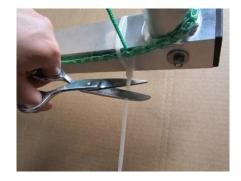
d) Cut the attached cord in half so that there are 2 short cords. Fix the end of one cord in one upper ring nut and knot it well. Pull the cord through the net meshes and fix it in the 2<sup>nd</sup> upper ring nut and knot it well. Repeat the steps with the 2<sup>nd</sup> cord in bottom ring nuts.
