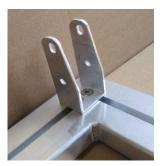
c) To fix the lower hinge stick from the bottom (upright's end) 1 nut 20 mm, M 8 each in the guide rail of the upright. Mount lower hinge with 1 fastening borehole.
