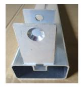
d) Beat cap 80 x 40 into the upright (use a mallet if necessary), adjust lower hinge and tighten fixing screw. Take care that the hinge at the bottom is flush with the upright's cap.
