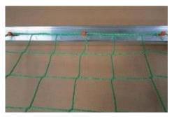
c) Dismantling of the net is also done by rotation of the net holders through 90 degrees. If necessary use a thin screw driver.
