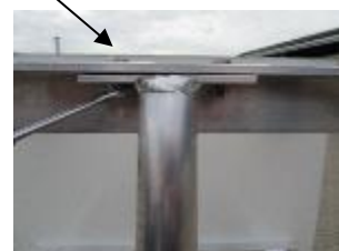
screw from the top hexagon screw M8 x20
